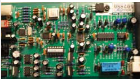
The Bryston BDA-1's D/A and output stages.
