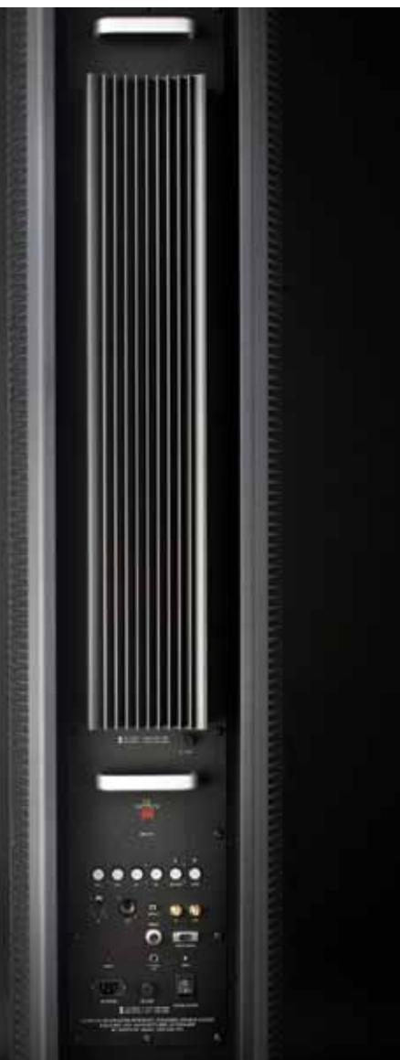
Specifications are as impressive as you'd expect at this level. Frequency response is a very wide 16Hz to 32kHz within a  $\pm 3\text{dB}$  envelope depending on Q setting. The Duelund topology crossover hands the bass drivers over to the mid ribbon at 250Hz which in turn hands over to the AMT array at 18kHz—yes, nigh on super-tweeter territory. Having such a wide bandwidth for the midrange promises continuity in tonal balance and reduced crossover artefacts.
