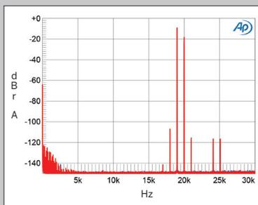
**Fig.14** Gryphon Ethos, Filter 4, HF intermodulation spectrum (DC–30kHz), 19+20kHz at OdBFS into 600 ohms (left channel blue, right red; linear frequency scale).
