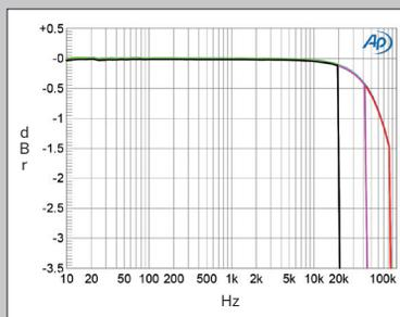
**Fig.8** Gryphon Ethos, Filter 7, frequency response at -12dBFS into 100k ohms with data sampled at: 44.1kHz (left channel green, right gray), 96kHz (left cyan, right magenta), 192kHz (left blue, right red) (0.5dB/vertical div.).
