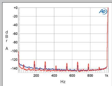
**Fig.9** Gryphon Ethos, spectrum with noise and spurs of dithered 1kHz tone at 0dBFS (left channel blue, right red) (20dB/vertical div.).
