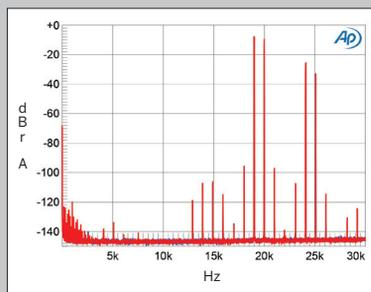
**Fig.13** Gryphon Ethos, Filter 1, HF intermodulation spectrum (DC–30kHz), 19+20kHz at OdBFS into 100k ohms (left channel blue, right red; linear frequency scale).
