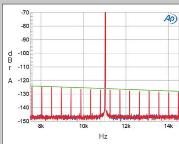
**Fig.15** Gryphon Ethos, high-resolution jitter spectrum of analog output signal, 11.025kHz at –6dBFS, sampled at 44.1kHz with LSB toggled at 229Hz: CD data (left channel blue, right red). Center frequency of trace, 11.025kHz; frequency range, ±3.5kHz.
