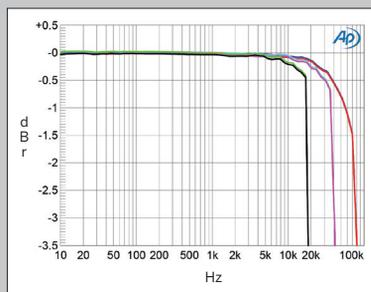
**Fig.7** Gryphon Ethos, Filter 4, frequency response at -12dBFS into 100k ohms with data sampled at: 44.1kHz (left channel green, right gray), 96kHz (left cyan, right magenta), 192kHz (left blue, right red) (0.5dB/vertical div.).
