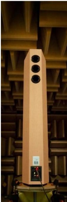
Our speaker design and manufacturing facility in Canada has a very unique advantage – an on-site ‘anechoic chamber’. Anechoic chambers are reflection free rooms and are used by the superior speaker manufactures to do all the loudspeaker testing in an environment where early reflections and outside noise issues are eliminated from the measurement curve(s). Anechoic chambers are very, very expensive to build but they are invaluable when designing a quality loudspeaker.
