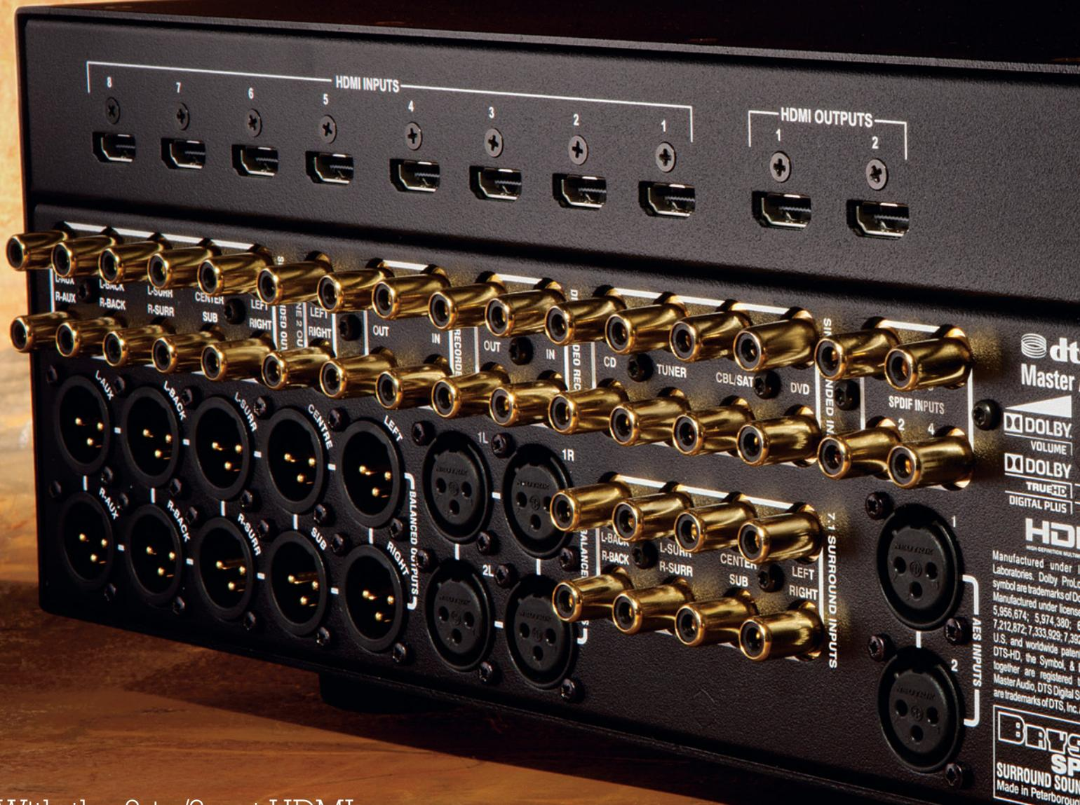
'With the 8-in/2-out HDMI's and fully-balanced XLR terminals, the rear panel is pure home cinema heaven'
